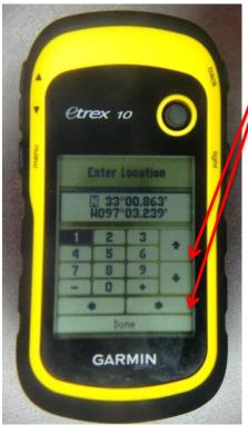
Moving around on the Coordinates screen is done by using up / down / left / right arrows.
